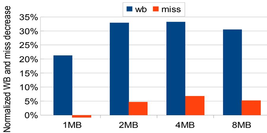
Fig. 12: Normalized Writebacks and Misses decrease under varied cache sizes, SPEC2006 (higher is better).
