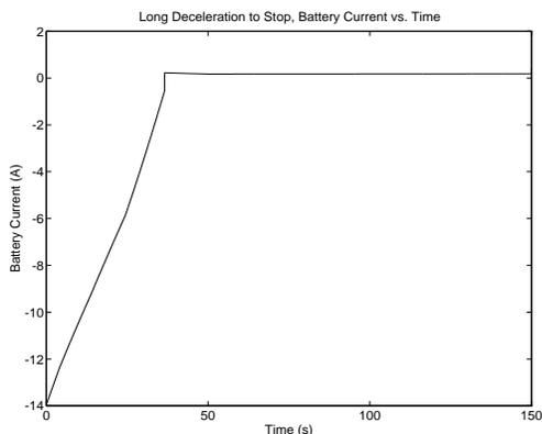
**Figure 3:** Long deceleration from stop, current.
