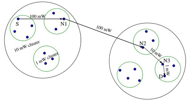
Fig. 4. Routing by CLUSTERPOW in a typical non-homogeneous network.
