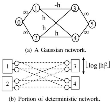
Fig. 2. Example showing that the linear deterministic model does not approximate the capacity of the Gaussian network to within a bounded number of bits.
