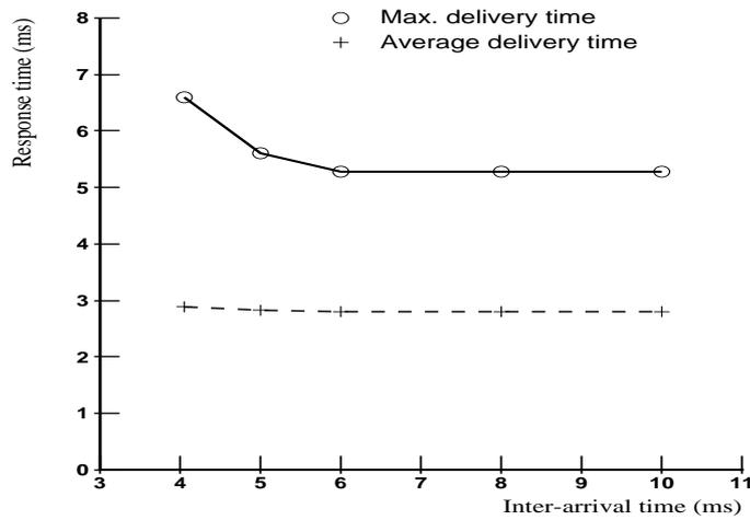
**Figure 12** Observed delays in a 4-dim. 256-node system.
