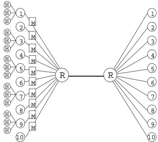
Figure 1: Simple topology for simulation with aggregated sources
