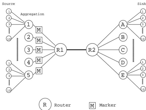
Figure 4: Aggregated network topology with different RTTs
