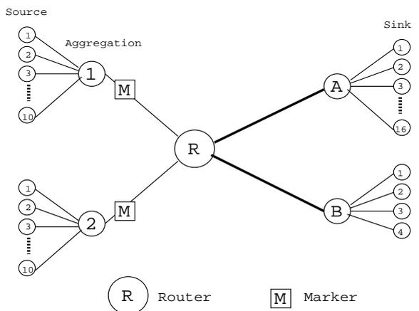
Figure 6: Aggregated network topology with different congestion levels
