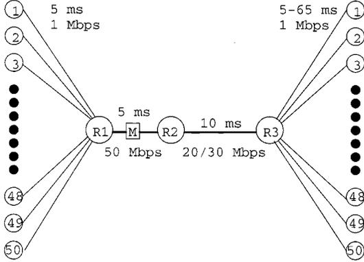
Fig. 16. Aggregated network topology with different RTTs.
