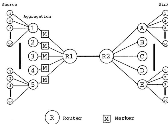
Fig. 19. Aggregated network topology with multiple aggregations.
