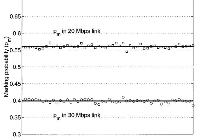
Fig. 17. The probability of a packet marked IN.
