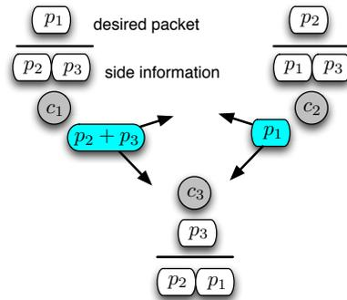
Fig. 1. Coded information exchange between clients  $c_1, c_2, c_3$ .
