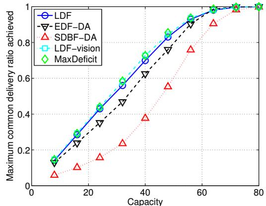
**Figure 5: Maximum common delivery ratio achieved with different capacities for  $\tau_{\max} = 2$ .**
